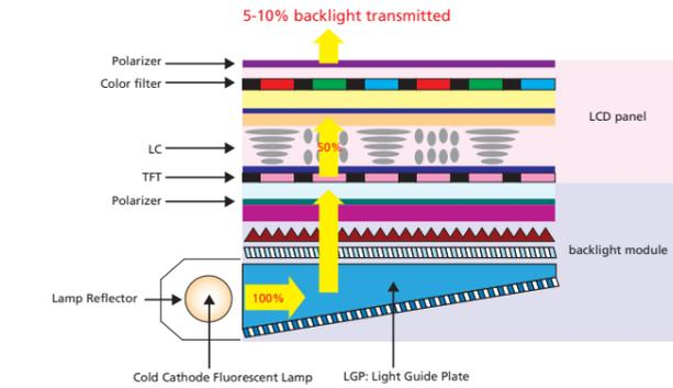
Brightness can be enhanced by improvements to the backlight module, TFT/ Color filter layout and LC systems.
