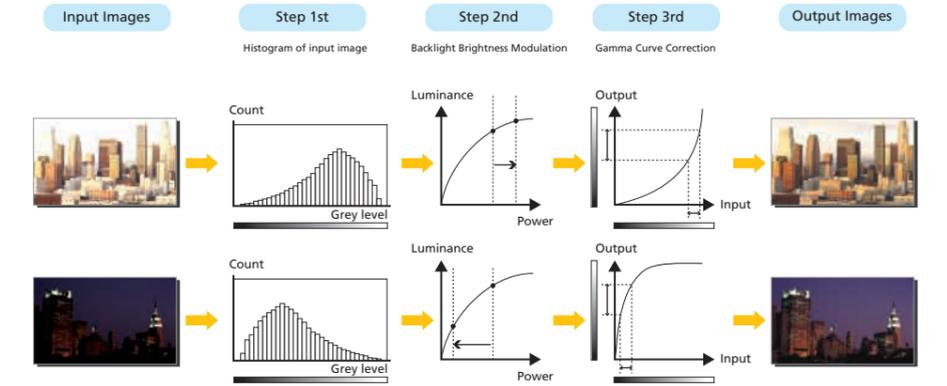
Dynamic adjustment of contrast ratio delivers drastic improvements because the adjustments affect the input image directly and therefore the full capability of the LCD panel can be realized -- images look ultra-sharp and power is used efficiently.
